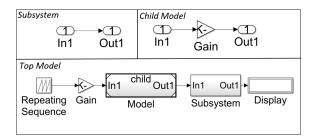
Figure 10: Bug TSC-02515280: For the child model (top right) Simulink's *Verification and Validation* toolbox API calculates inconsistent *SubSystemCount* values. MathWorks ruled the API specification ambiguous, as it did not properly define the API's scope.
