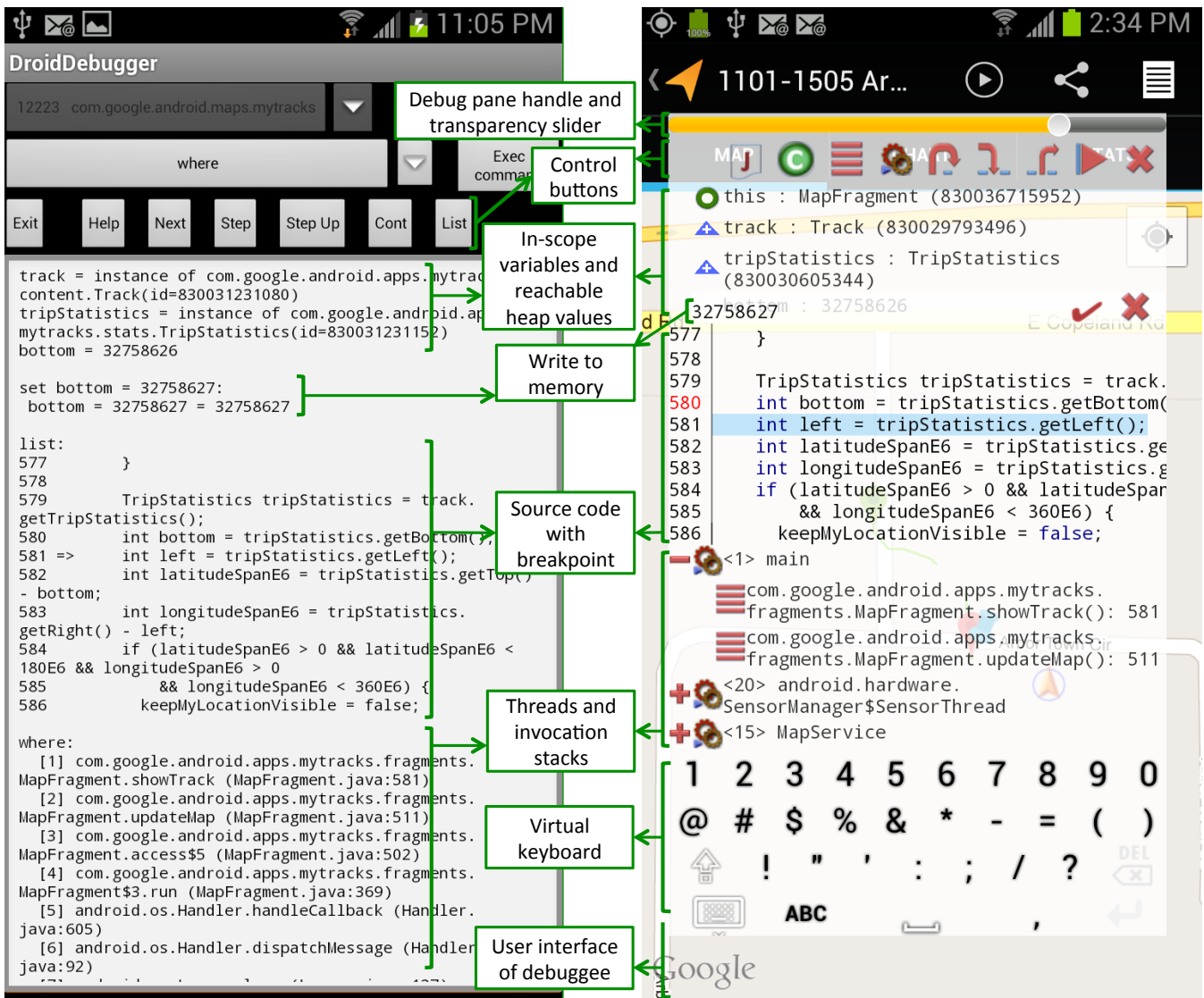
Fig. 2. DroidDebugger (left) and GROPG (right) while debugging the My Tracks application on a Samsung Galaxy S3 phone. In both cases the programmer set a breakpoint at line 580 of the MapFragment class. After My Tracks stopped at the breakpoint, the programmer stepped to line 581, inspected in-scope memory values, and updated the local variable named bottom.
