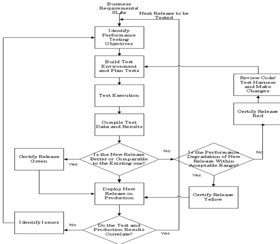
Figure 2: Performance Testing Workflow Extended with Release Certification and Data Correlation Components
