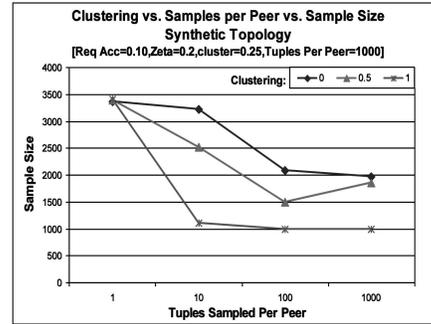
Fig. 17. Effects of clustering with the number of tuples sampled per peer on the sample size by using the *AVERAGE* technique for synthetic topologies.
