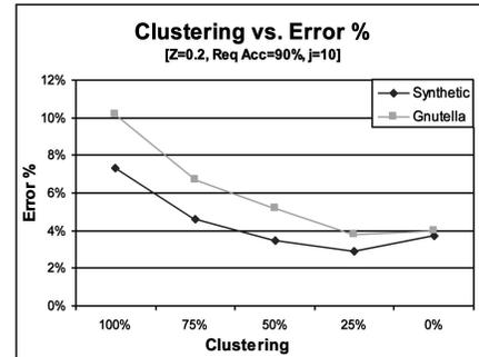
Fig. 19. Effects of clustering on the error percentage for the *MEDIAN* technique.
