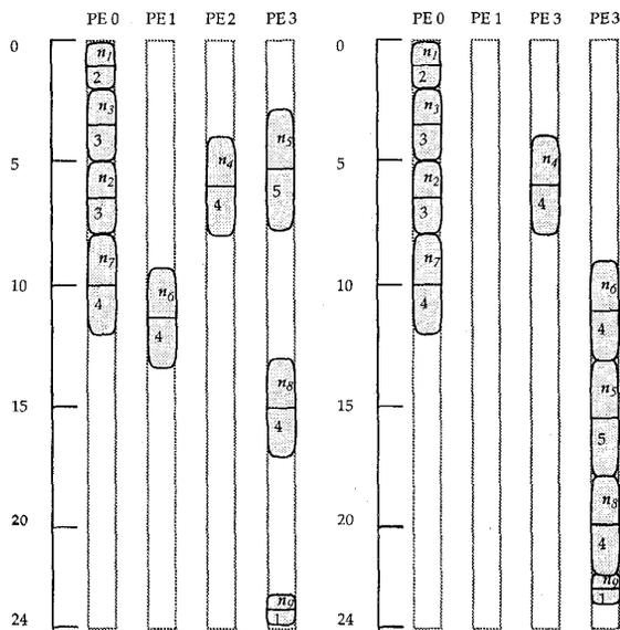
Figure 4: (a) Schedules generated by the *InitialSchedule()* (schedule length = 24); (b) The final schedule after the local search process with node  $n_6$  is transferred to PE 3 (schedule length = 23).
