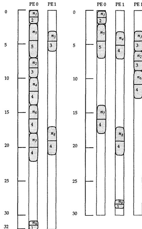
Figure 2: Schedule generated by (a) the MD algorithm (schedule length = 32); (b) the ETF and DLS algorithm (schedule length = 29).
