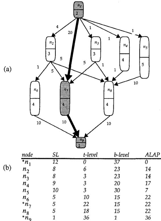
Figure 1: (a) A task graph; (b) The static levels (SLs), *t-levels* (ASAP times), *b-levels*, and ALAP times of the nodes (CPNs are marked by an asterisk).
