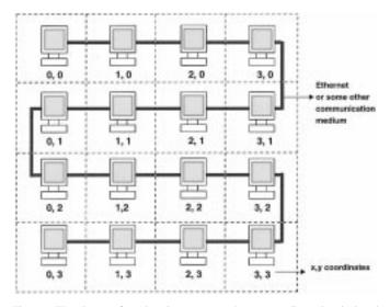
Fig. 1. The cluster of workstations connected as a two-dimensional virtual topology.
