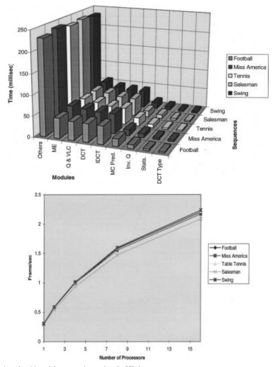
Fig. 4. Comparison of modules and frame processing speed on the SGI cluster.
