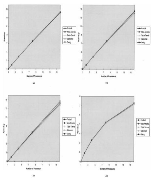
Fig. 3. Speedup of (a) motion estimation, (b) DCT, (c) quantization and VLC and (d) overall speedup on the SGI cluster.
