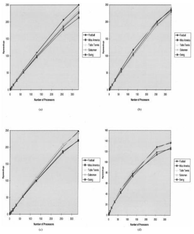
Fig. 5. Speedup of (a) motion estimation, (b) DCT, (c) quantization and VLC and (d) overall speedup on the paragon.
