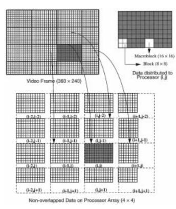
Fig. 2. Distribution of a frame on the virtual network topology.
