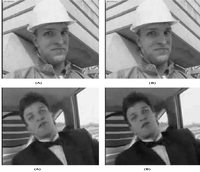
Fig. 4. Coded video quality comparison for Frame 150 of “Foreman” and Frame 80 of “Carphone” when (a) 100% blocks are encoded and (b) 20% blocks are encoded.
