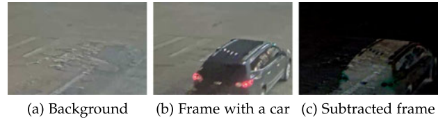
Fig. 3. An example of SDD. The subtracted frame highlights the car that entering the scene.
