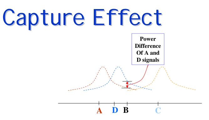
A and D transmit simultaneously to B, the signal strength received by B from D is much higher than that from A, and D's transmission can be decoded without errors. This will result unfair sharing of bandwidth.
