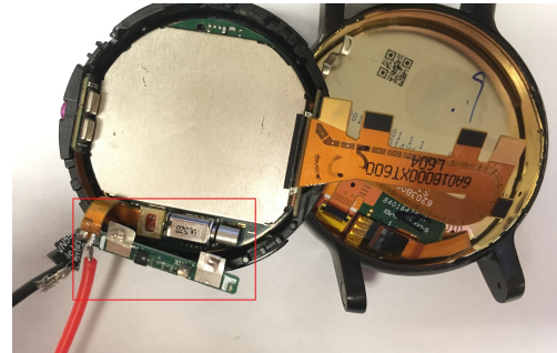
Figure 11: Power measurement of an Moto 360 smartwatch. A compatible battery interface circuit (as shown in the red box) was carved out from the same smartwatch and used as an adapter between the watch and the power monitor.
