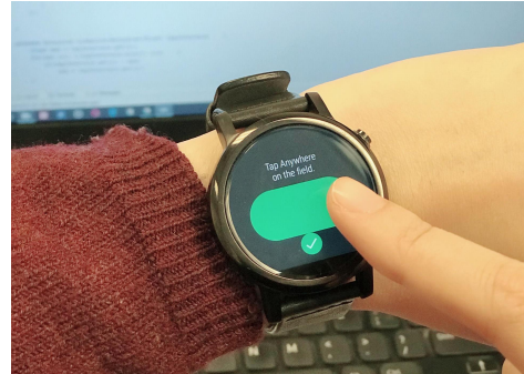
Figure 1: The prototype of Beat-PIN that we develop for the smartwatch. A beat-PIN is characterized by the timing of its beats.
