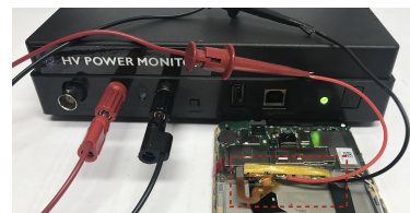
Fig. 14. Power measurement of a Huawei Honor smartphone. A compatible battery interface circuit (as shown in the red box) was carved out from the same smartphone and used as an adapter between the phone and the power monitor.
