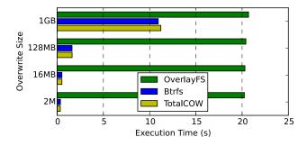
Figure 6: Overwrites with various data sizes on a 1 GB file
