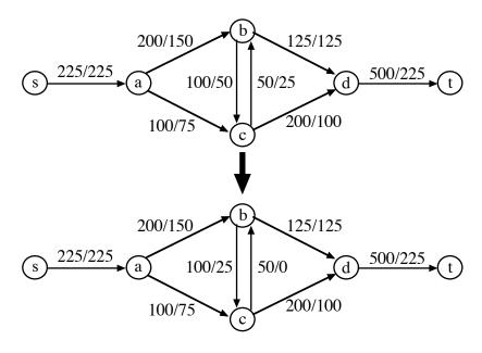
Solution is *not optimal* if an "augmenting path" (A.P.) from the source to sink can be found.
