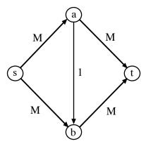
Can lead to 2M A.P.s that each contribute one unit of flow.
