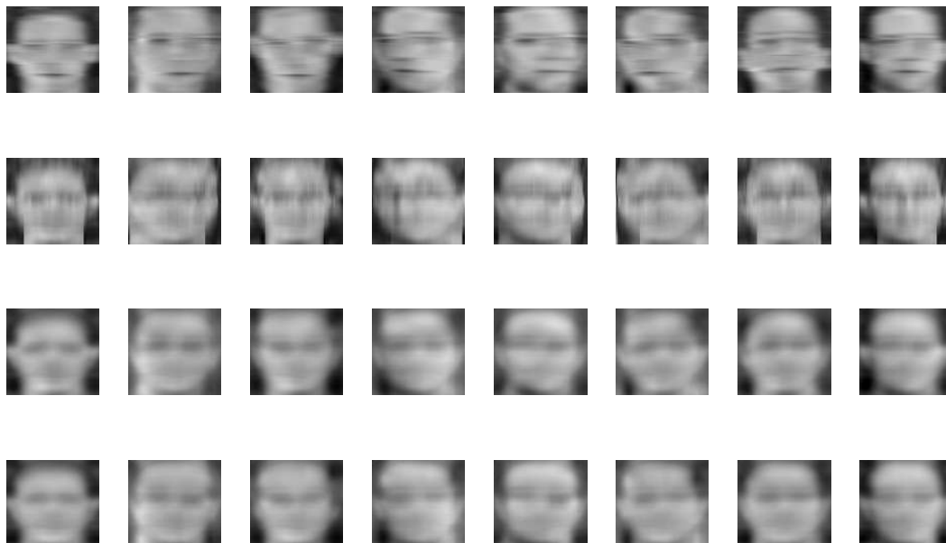
Figure 1: Reconstructed images by 2dLRi (first row), 2dLiR (second row), 2DSVD (third row), and LMR (fourth row) on ORL dataset at k = s = 5 .
