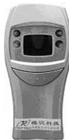
Fig.10. Hand-held iris sensor.
