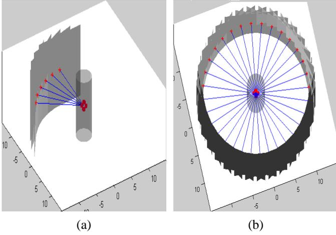
Fig. 5. Setting up projection plane geometry for images taken from different views. (a) some example views for consecutive images. (b) all views forming a full circle.
