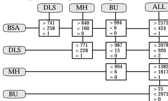
Figure 4: A comparison of the APN scheduling algorithms in terms of better, worse and equal performance across all topologies.
