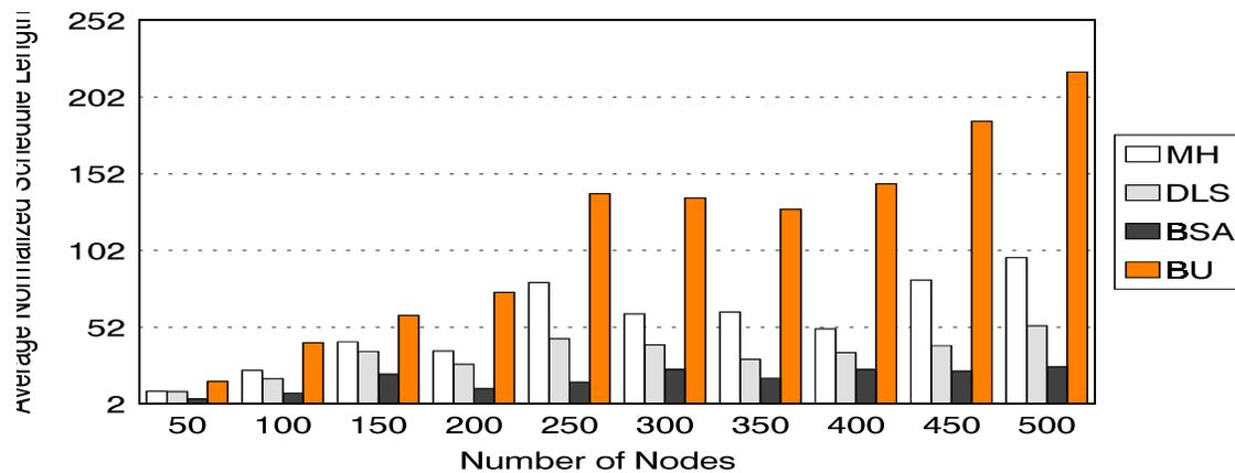
Figure 2: The average normalized schedule lengths produced by the APN scheduling algorithms for task graphs of various sizes on a 8-node hypercube.
