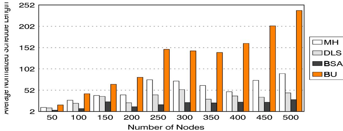
Figure 1: The average normalized schedule lengths produced by the APN scheduling algorithms for task graphs of various sizes on a 4x2 mesh.
