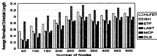
Figure 2: The average normalized schedule lengths produced by the BNP scheduling algorithms for task graphs of various sizes given only 50% of the average number of processors.
