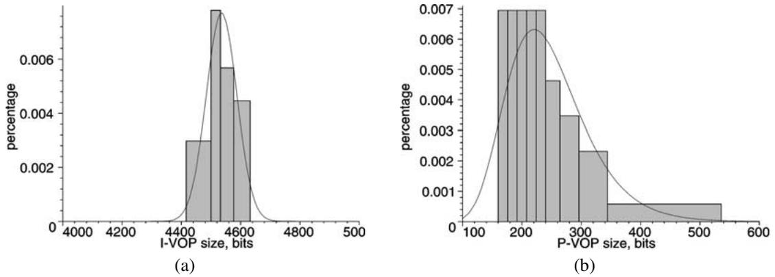
Figure 2. (a) I-frame size distribution; (b) P-frame size distribution.
