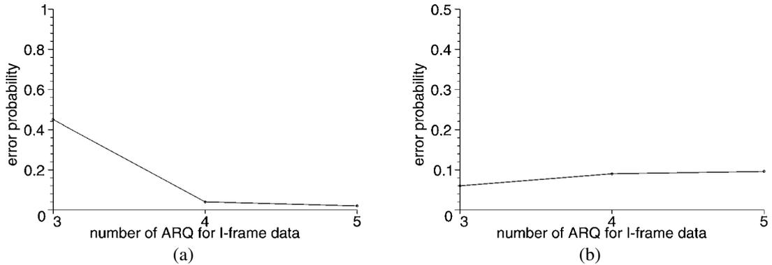
Figure 10. Average packet error rate (I-frame ARQ = 3, 4, 5; P-frame ARQ = 3 only). (a) I-frame error rate; (b) P-frame error rate.
