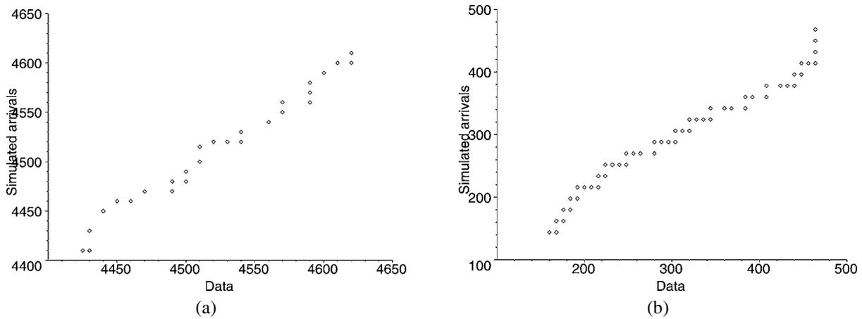
Figure 6. QQ plots for trace data and simulated arrival data. (a) For I-frame arrivals; (b) for P-frame arrivals.
