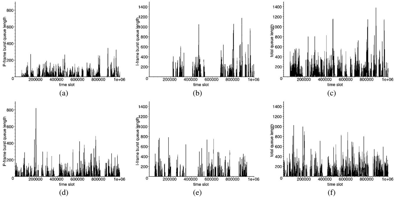
Figure 7. Comparison of the queue length dynamics. (a) P-frame bursts, FIFO case; (b) I-frame bursts, FIFO case; (c) total queue, FIFO case; (d) P-frame bursts, priority case; (e) I-frame bursts, priority case; (f) total queue, priority case.
