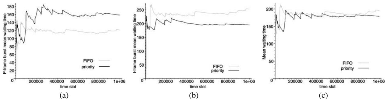
Figure 8. Comparison of the mean waiting time. (a) For P-frame bursts; (b) for I-frame bursts; (c) for all RLC bursts.
