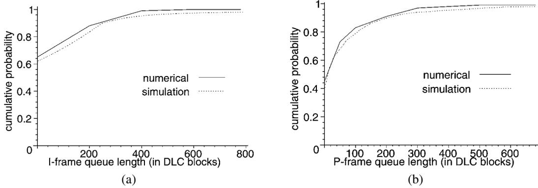
Figure 4. Comparison of the queue length distribution: numerical vs. simulation.
