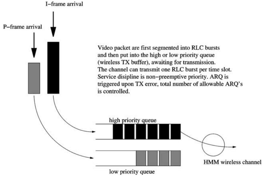
Figure 3. A diagram of DBMAP/PH/1 with priority queueing system.
