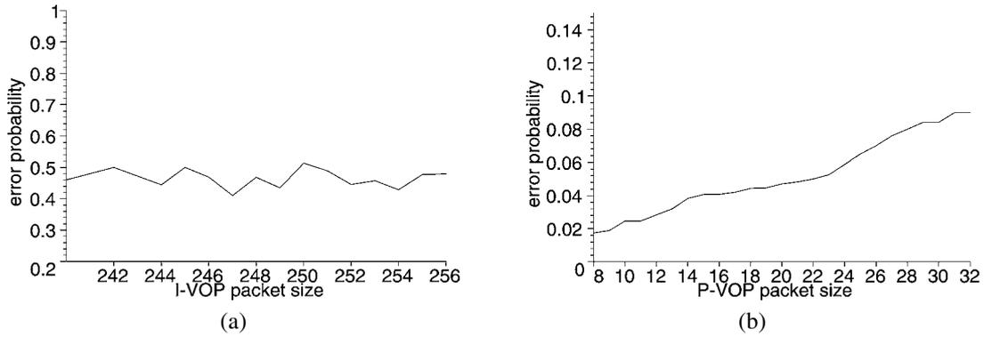
Figure 9. Packet error rate vs. packet size (both I-frame and P-frame ARQ = 3). (a) I-frame error rate; (b) P-frame error rate.
