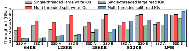
Figure 5: Throughput of single-threaded large aligned IOs vs. multi-threaded split 32KB aligned IOs. SSD A: the PCIe4.0 SSD [59]. SSD B: the PCIe5.0 SSD [58].
