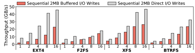
Figure 1: Maximum performance of direct I/O via a RAID0 array with 8 PCIe4.0 SSDs [51] (about 55GB/s total bandwidth) and buffered I/O via 8 DDR4 DRAM (about 200GB/s total bandwidth) under different thread counts.
