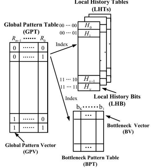
Fig. 2. The structure of the two-level predictor.
