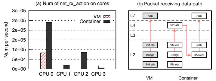
Fig. 13: Software interrupt distribution among multi cores and network data path in VMs or containers.
