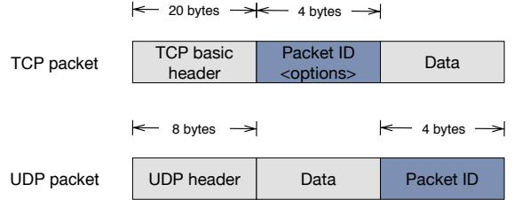
Fig. 3: Add unique packet ID into network packets.
