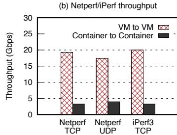
Fig. 12: Container multi-host networking setting and the Netperf/iPerf throughput of VMs versus containers.
