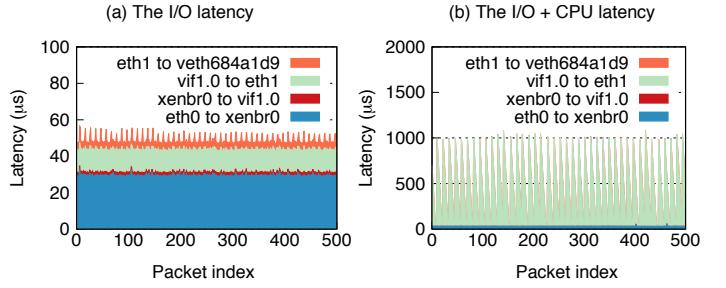
Fig. 11: Latency decomposition when the Sockperf VM runs alone or shares the physical CPU with a CPU-bound VM.
