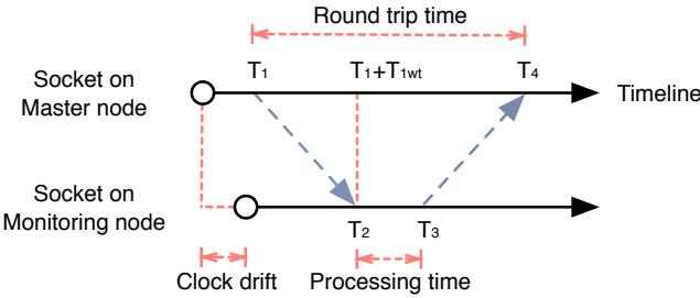
Fig. 4: Calculating the clock drift between two machines under the Cristian’s algorithm [29].
