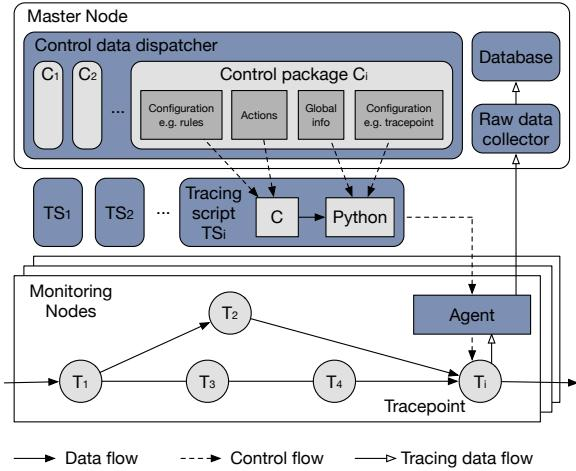
Fig. 2: vNetTracer architecture.
