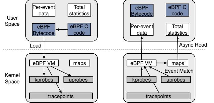
Fig. 1: The mechanism of eBPF in Linux. The left one shows the eBPF code insertion from user space into kernel space. The right one shows the trace data is collected from kernel space to user space when eBPF programs execute.
