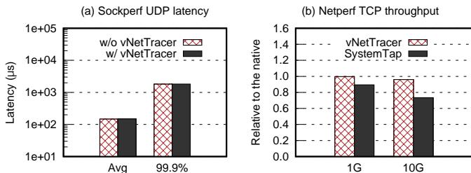
Fig. 7: vNetTracer incurs negligible overhead to (a) application average latency, tail latency, and (b) throughput. Compared to SystemTap, the overhead is marginal due to the eBPF benefits and the optimizations to vNetTracer.
