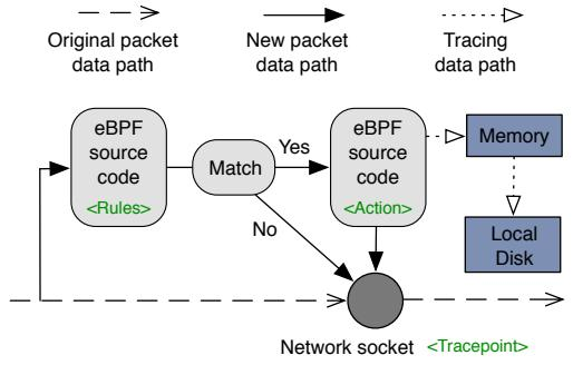
Fig. 5: How eBPF code works for packet filtering and tracing.
