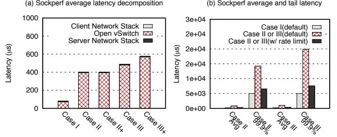
Fig. 9: Open vSwitch latency decomposition and analysis.
