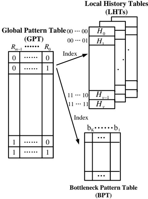
Fig. 4. The structure of the two-level predictor.
