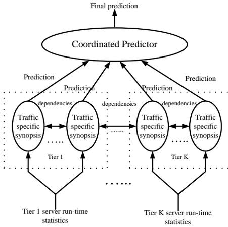
Fig. 3. The two-level coordinated prediction framework.
