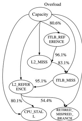
Fig. 6. Bayesian Network structure for hardware counter metrics.
