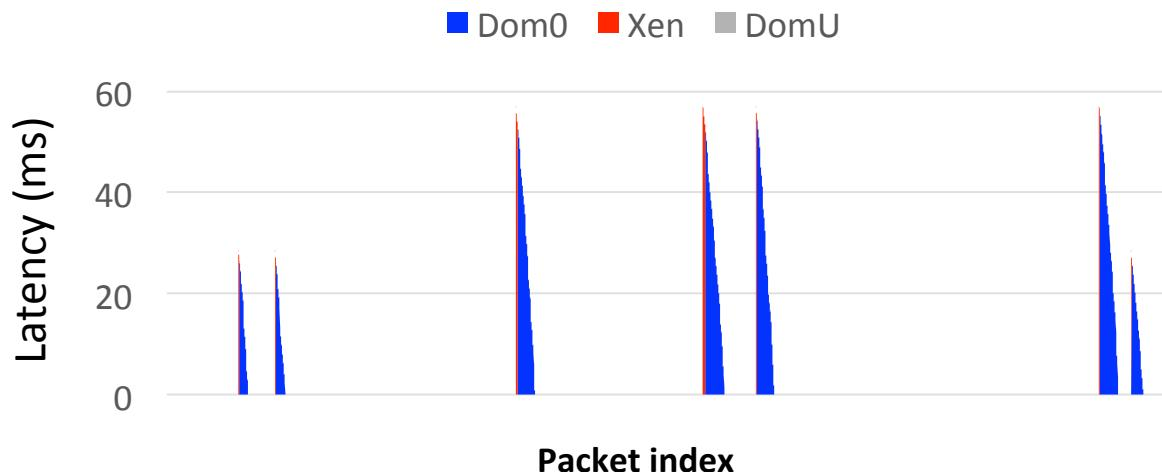
**BUG-2: Xen does not timely activate I/O VMs that are deactivated due to long idling**
