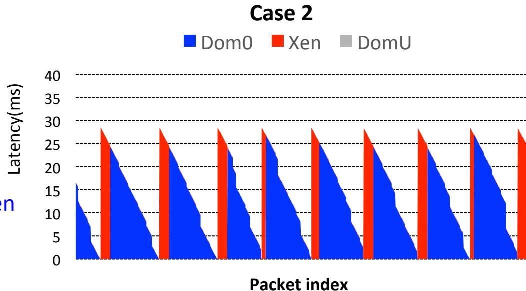
**BUG-1:Xen mistakenly boosts the priority of CPU-intensive VMs, which causes long scheduling delays of the I/O-bound VM in Xen**
