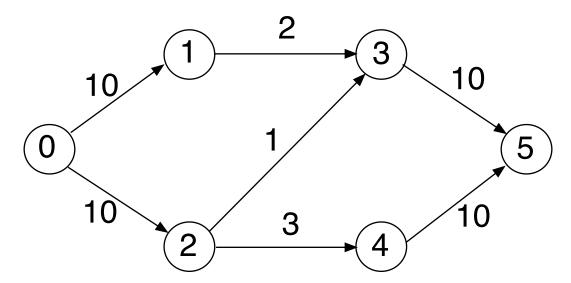
What is the maximum flow for this network? 0 is the source and 5 is the sink.
