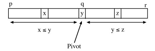
Customarily, the last subarray element (subscript r) is used as the *pivot* value.
